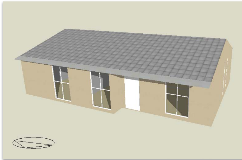
Figure 10-9: Geometry of the 3D DesignBuilder model of the original pre-retrofitted fibro house used for thermal analysis.
